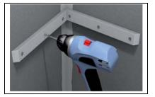
Mount the brackets through the wedi Building Panel wall into the solid 2' x 4' wooden framework.
