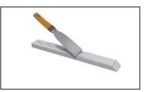
Evenly distribute wedi Joint Sealant with a putty knife until the whole contact area is covered.
